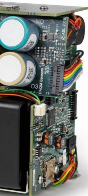
The AS330 metal oxide sensor management system provides precise management of 8 metal oxide sensors.
