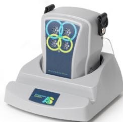
In many circumstances a wearable air quality monitoring system that also makes use of a complementary range of sensing technologies will be the optimum way to provide a reliable information set: Electrochemical, NDIR, and metal oxide sensors can all be included in the system, as can motion detection (3-axis accelerometer and GPS), together with ambient noise, temperature and relative humidity measurement.
